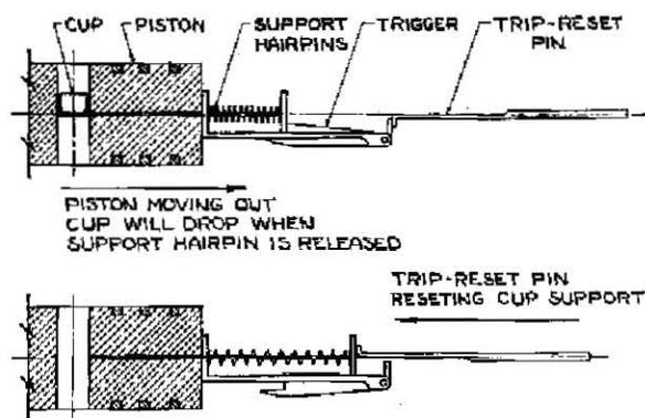
Fig. 2 Operation of trip and reset mechanism
