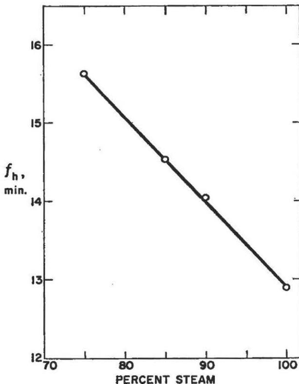
Fig. 3. Heating rate of water in quart jars in 165° F. steam-air mixtures.
