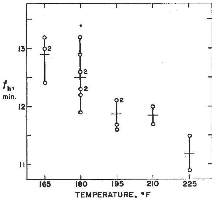
**Fig. 1.** Slope of the heating curve ( $f_h$ ) of quart jars of water in saturated steam.
