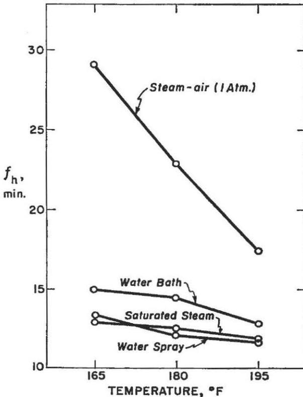
Fig. 5. Average heating rate of water in quart jars as a function of temperature.
