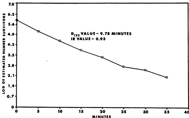
FIG. 1. Survivor curve for spore K-3-110 that was heated at 125°C at an ambient relative humidity of 50%.
